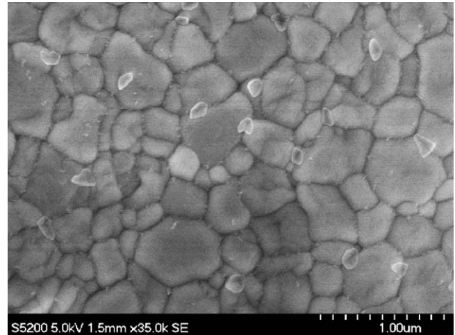
Fig. 1. HRSEM micrograph of polished and thermally etched cross-section of as-fabricated BaCe 0.95 Y 0.05 O 3-δ polycrystal.
